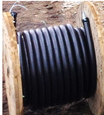
Figure 11. PVC-sheathed armoured cable on a spool
